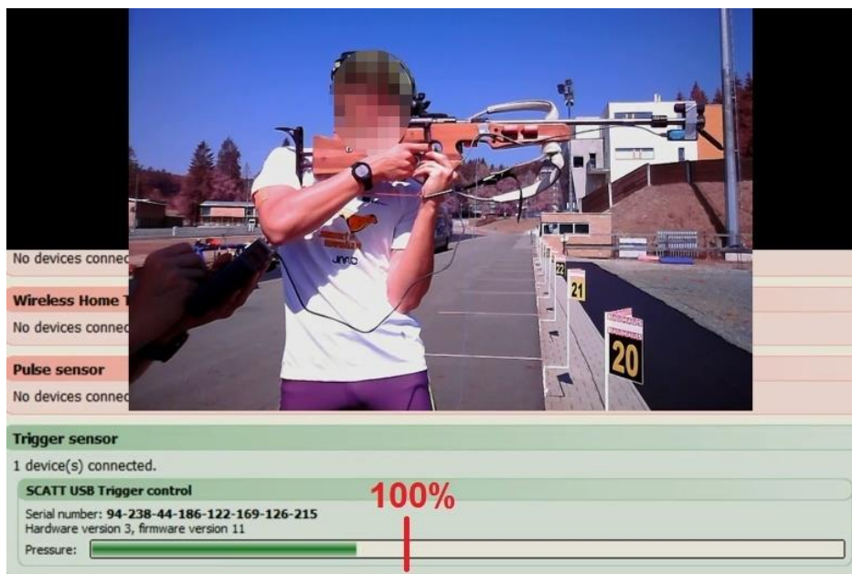
Figure 2. Pressure measuring on the trigger during shooting.
