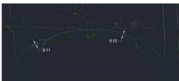
Figure 15: Point cloud section during the restoration works. The measure of the vault section can be obtained.
