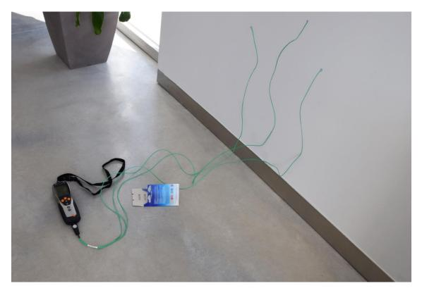
Figure 6. Measurement of *U* thermal transmittance of the opaque house enclosure; 11 April 2019, 5 pm.
