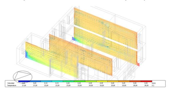
Figure 13. Simulated (CFD) of the house's thermal behaviour; 1 August 2018, 3 pm.
