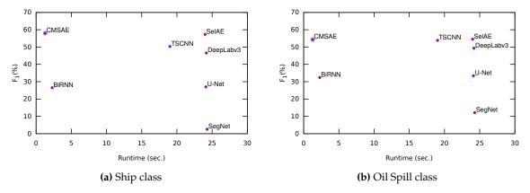
**Figure 10.** Comparison of the result obtained from a Multi-objective Optimization Problem (MOP) perspective, comparing the result of the classification and the runtime for the ship and oil spill classes.
