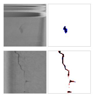
**Figure 9.** Results of processing two SLAR input images with the proposed method (zooming in the area of interest). The first column shows the original SLAR images and the second column shows the detection results. Black areas depict correct detections of oil spills, red and blue pixels depict FP and FN of oil spills, respectively, and white pixels represents correct detections of the background.
