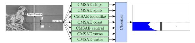
**Figure 3.** Architecture of the proposed network. Each scanline is supplied to a series of ConvLSTM Selectional AutoEncoders (CMSAE) networks to process each of the different classes in parallel. The results of these networks are given to a final classifier which performs the prediction.
