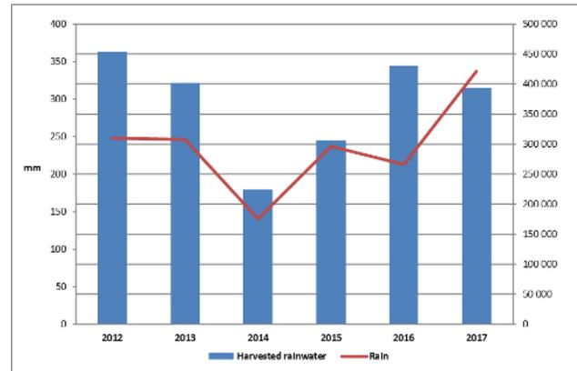
**Figure 3:** Volume of harvested water in the anti-pollution tank and rainfall (2012-2017). Water collected in 2011 is not included in this chart since the tank started operating in May 2011 so as not to disturb the analysis period (annual). *Source: the Authors.*
