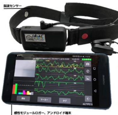
Figure 2. Band-type EEG and KANEI module logger
