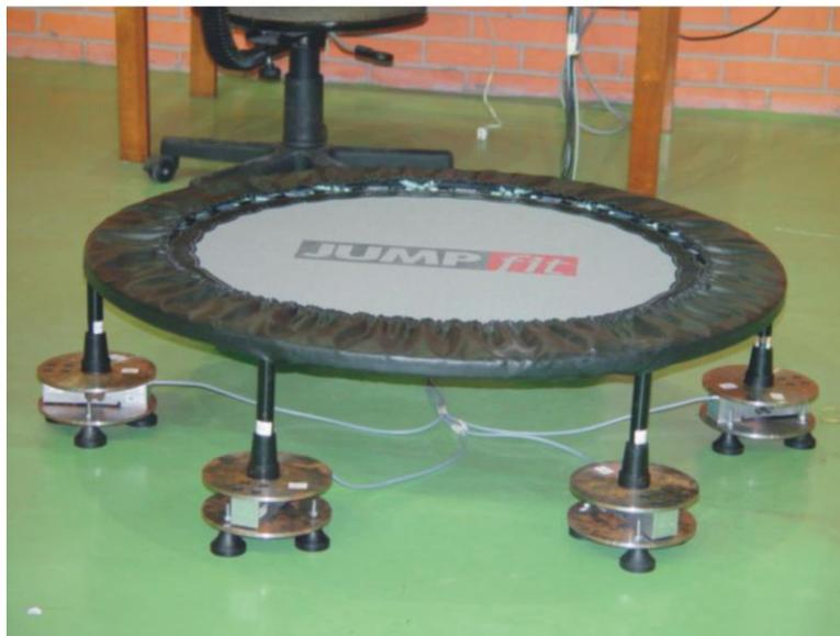
Figure 1. Rebound exercise mini-trampoline with attached load cells
