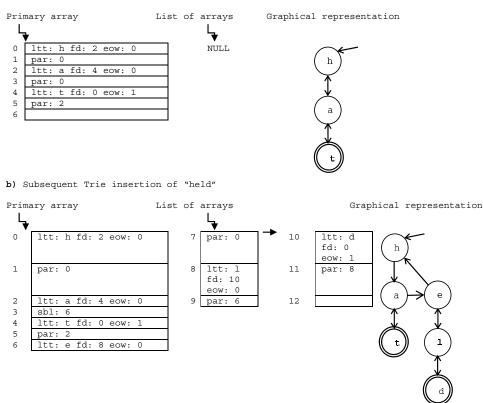
**Figure 1.** Sequential and graphical representations of Trie (ltt: letter; fd: first descendent index; eow: end of word; par: parent index; sbl: sibling index; BN0 = 7; BN = 3) that indexes the terms *hat* and *held*.
