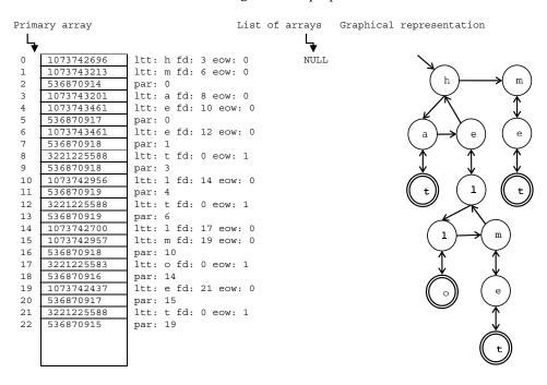
**Figure 3.** Trie with terms and identifiers: hat (8), hello (17), helmet (21) and met (12). (ltt: letter; fd: first descendent index; eow: end of word; par: parent index; sbl: sibling index; BN0 = 23; BN = 5).
