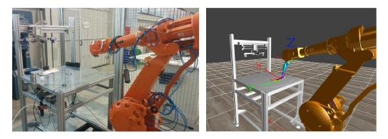
Figure 9. a) Shoe sole application with laser scanner. b) Shown in the simulator.
