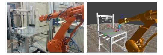
a) Shoe sole application with laser scanner. b) Shown in the simulator.
