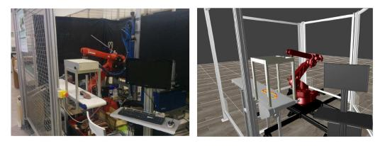
Figure 10. a) Shoe sole application with hot-melt. b) Shown in the simulator.
