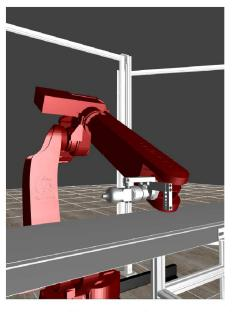
Figure 14. Monitoring the dangerous pose with the simulator in real-time.
