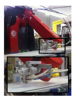
Figure 13. Robotic arm in a dangerous pose after following an incorrect normal.
