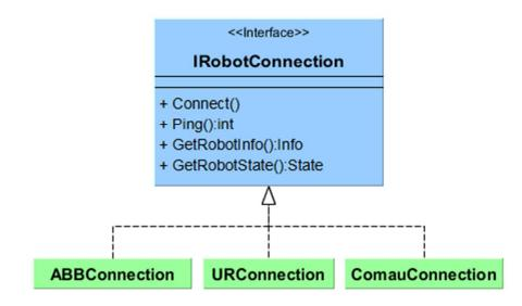
Common interface of the homogeneous connection model.
