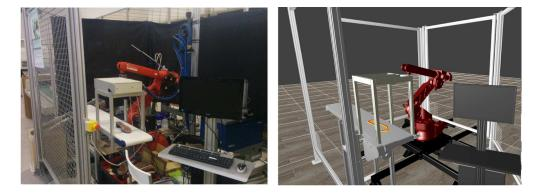
a) Shoe sole application with hot-melt. b) Shown in the simulator.
