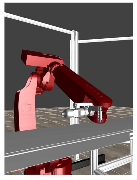
Monitoring the dangerous pose with the simulator in real-time.
