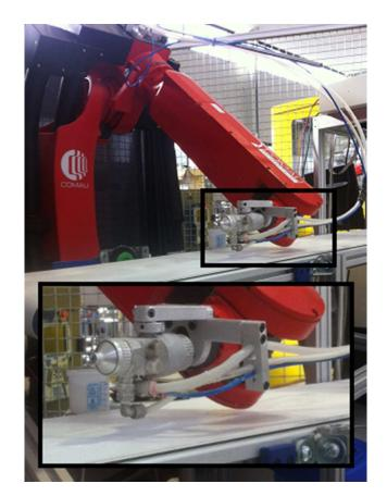
Robotic arm in a dangerous pose after following an incorrect normal.
