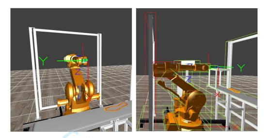
Figure 4. a) Collision hidden by perspective. b) Shown from another camera angle
