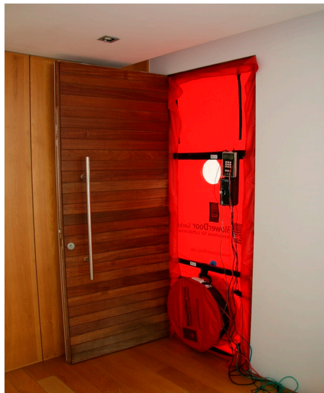
Figure 19. The blower door test. June 2015.
