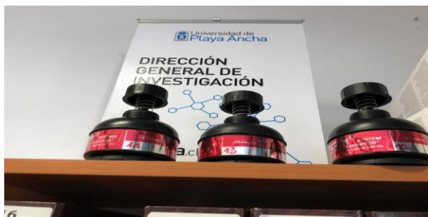
Fig. 3: Image of the Ionic Chamber of Electrete Placed in One of the Zones of Measurement.
