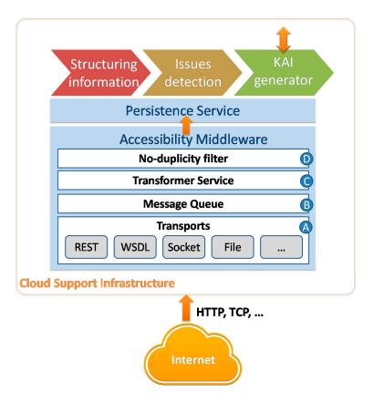
Figure 5. Components of the Cloud Support Infrastructure.
