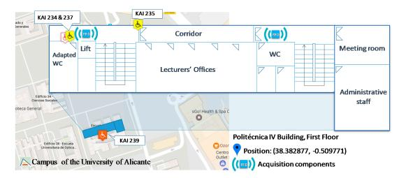
Figure 14. Indoor scenario and RFID-based acquisition components deployed.
