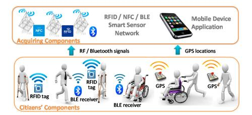
Figure 2. Acquisition infrastructure deployment.
