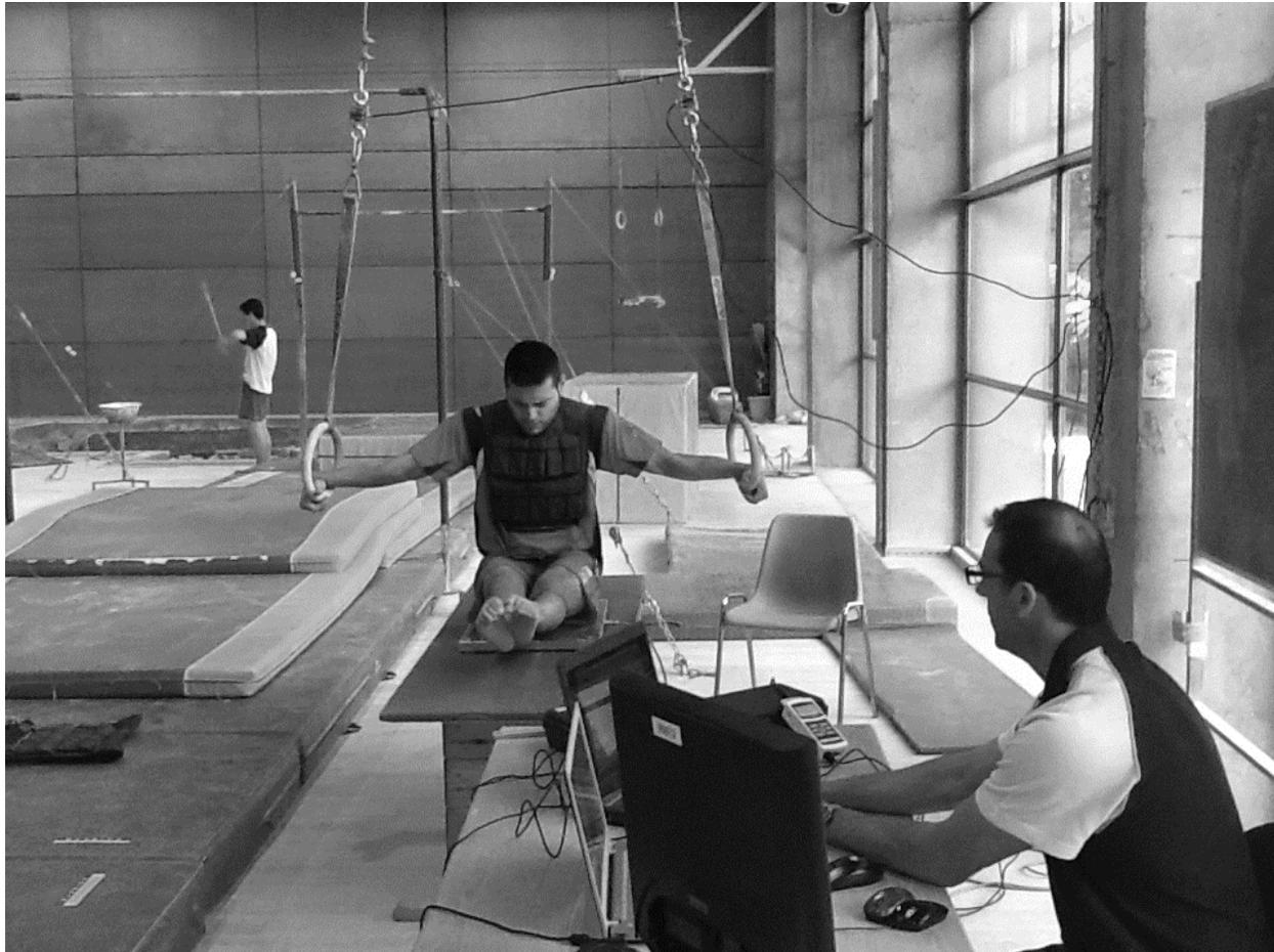
Figure 2. The initial position of the gymnast on the force platform and the hold of the rings without applying force.
