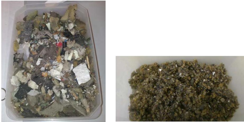
**Figure 1.** ASR before and after being crushed.
