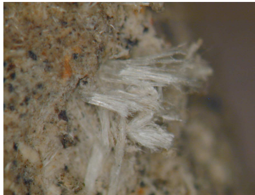
Figure 3. Chrysotile (micrograph of a sample of the roof of the Central Market, corresponding to a square plate of thickness 3 mm).
