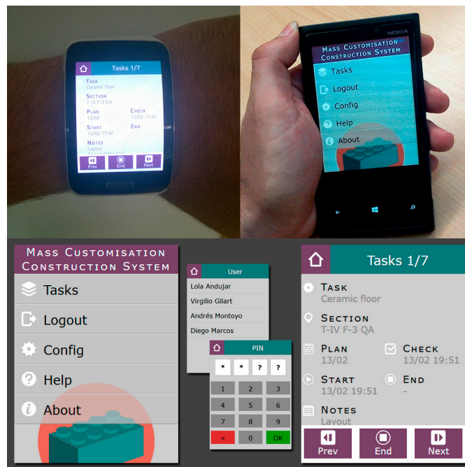
Figure 11. User agent for system interaction. Smartwatch and smartphone versions and interface screenshots.
