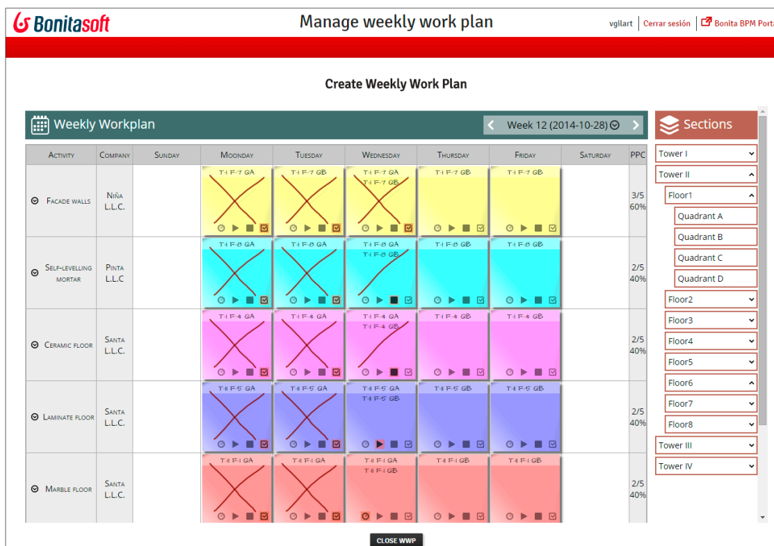
Figure 12. Screenshot of Weekly Work Plan application embedded in Bonita BPM. Traceability phase.
