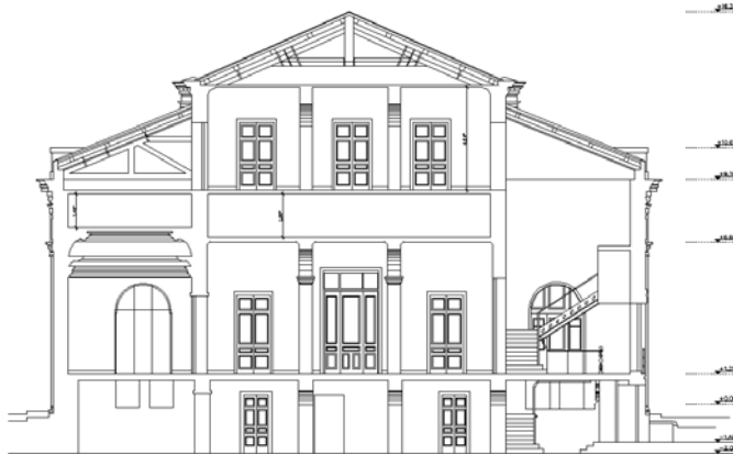
Fig. 3. Longitudinal section. North view. Wooden floor location (Saint James building Corfu Greece)
