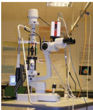
Fig. 1. Slit-lamp and digital video camera used to capture the images of frontal corneal.
