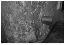
Figure 1: Ultrasonic Velocity Test, with an "Ultrasonic Tester", on a Concrete Reinforced Element Under Investigation
