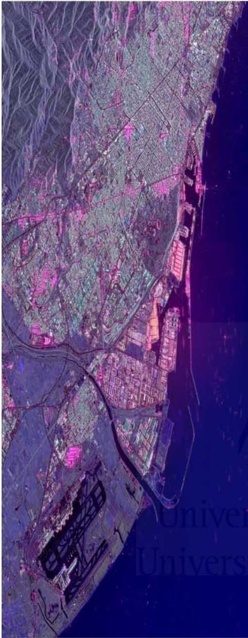
Fig. 3. Composite RGB image of the area under study in Barcelona (Spain) formed by the average intensities. Channels: R = HH - VV , G = 2HV , and B = HH + VV .
