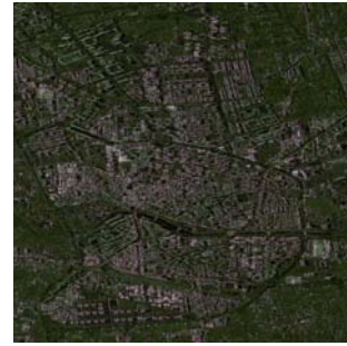
Fig. 1. Composite RGB image of the area under study in Murcia (Spain) formed by the average intensities. Channels: R = HH, G = VV, and B = HH - VV.
