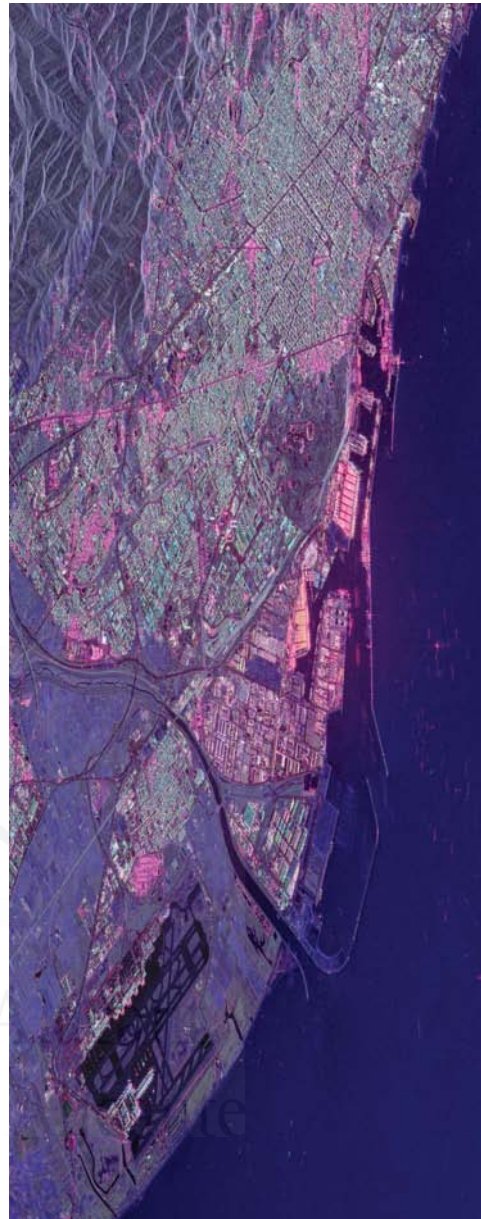
Fig. 1. Composite RGB image of the area under study in Barcelona, Spain, formed by the average intensities. Channels: R = HH - VV , G = 2HV , B = HH + VV
