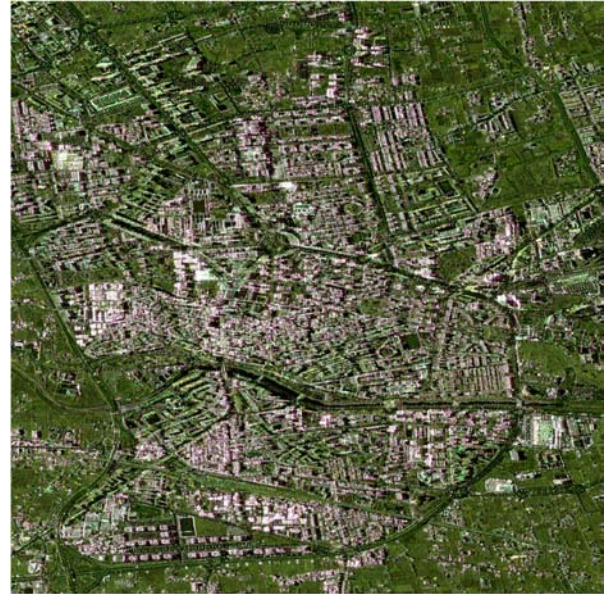
Fig. 4. Composite RGB image of the area under study in Murcia (Spain) formed by the average intensities. Channels: R = HH , G = VV , and B = HH - VV .
