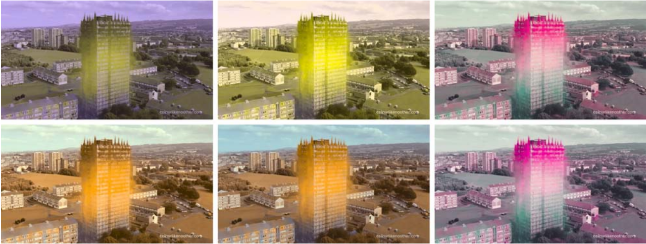
FIG. 3. From left to right, simulation of the perception of protanopic, deuteranopic and tritanopic subjects of the image shown at the upper-left part of the screen-shot in Figure 2. Results obtained with Boynton's (top row) and Guth ATD95 (bottom row) models.
