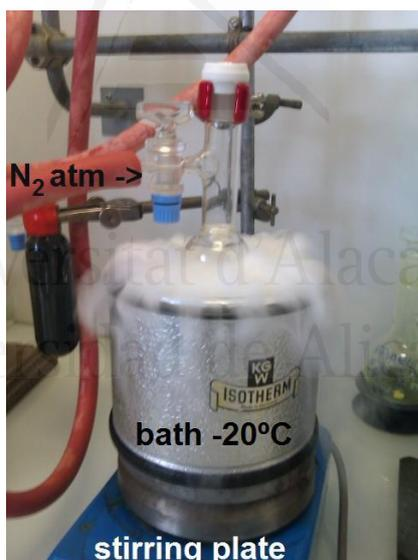
Figure 6.19. Photography of an intermediate step in the synthesis of the chiral R-BPPM ligand.
