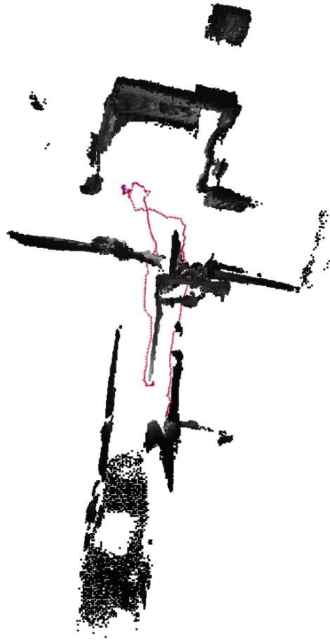
Figure 9: Planar based 6DoF egomotion results using planar patches after computing a GNG mesh.
