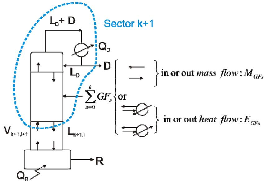
Figure 2. Generalized scheme of a distillation column.
