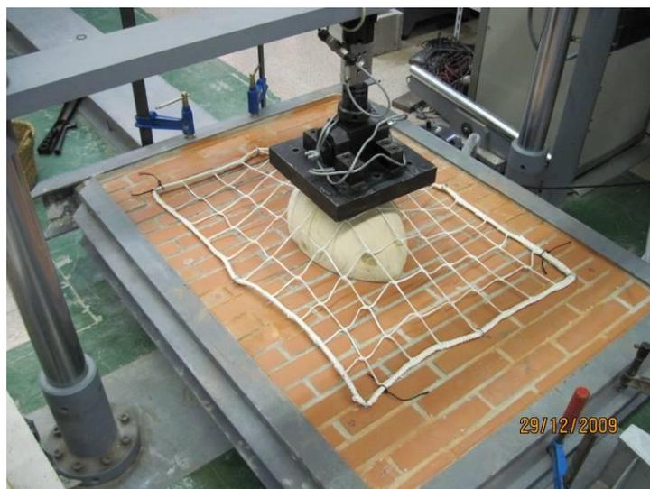
Figure 3: Stiff metal frame and wooden truncated ovoid.
