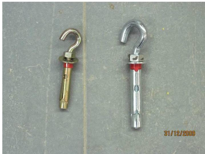
Figure 4: Metal anchors used in full scale tests.
