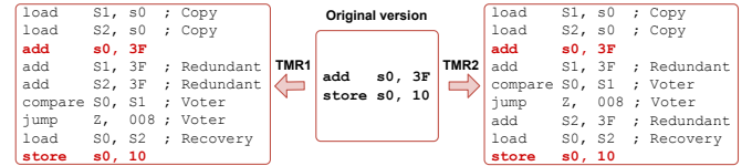
Figure 7: Hardened program using TMR1 and TMR2
