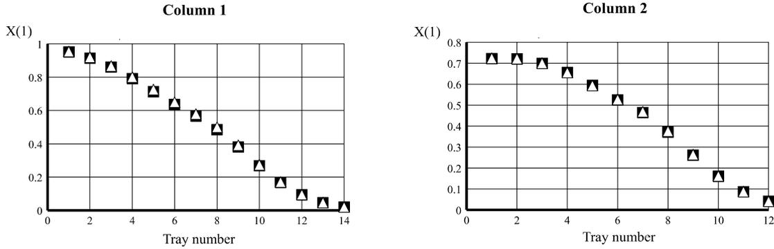
**Figure 11.** Results for column 1 and 2, comparing the approximate method ( $\Delta$ ) using the proposed correlation (Eqn. 14) and intersection with fitting of enthalpies (Eqns. 15 to 17) and the rigorous method ( $\blacksquare$ ).
