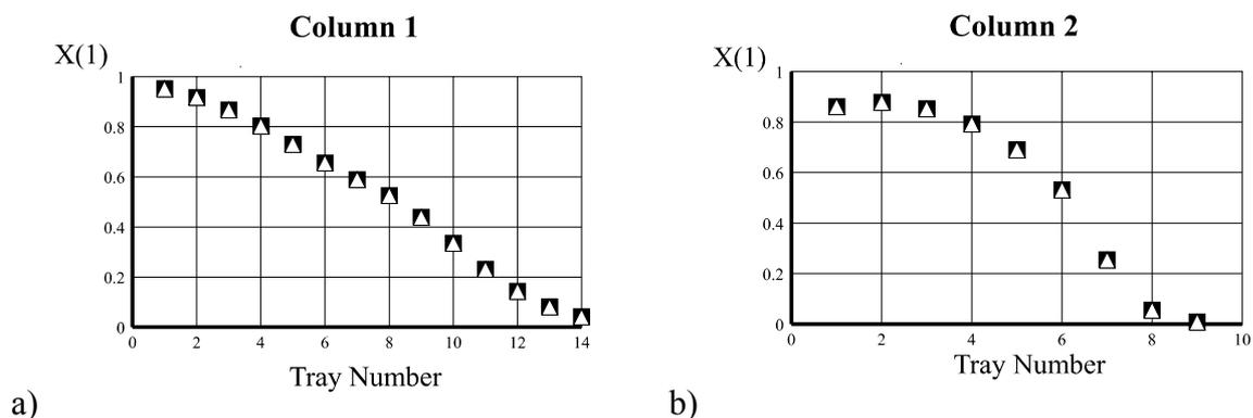
**Figure 9.** Comparison between the composition profiles obtained for component 1 in the liquid phase, by the rigorous design method proposed in present work (■) and by the Renon et al.<sup>13</sup> simulation method (Δ), for cases 1 (a) and 2 (b).
