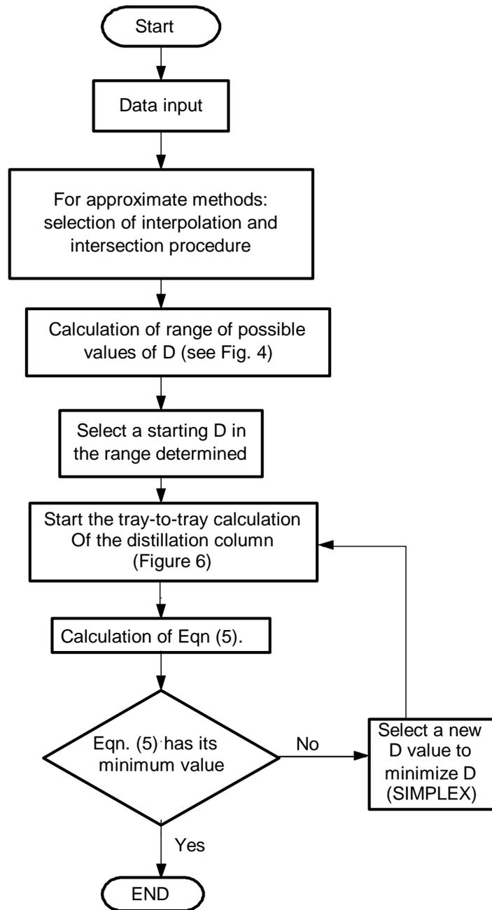
**Figure 8.** Flowsheet of the program to calculate a rectification column optimising the distillate flow rate.
