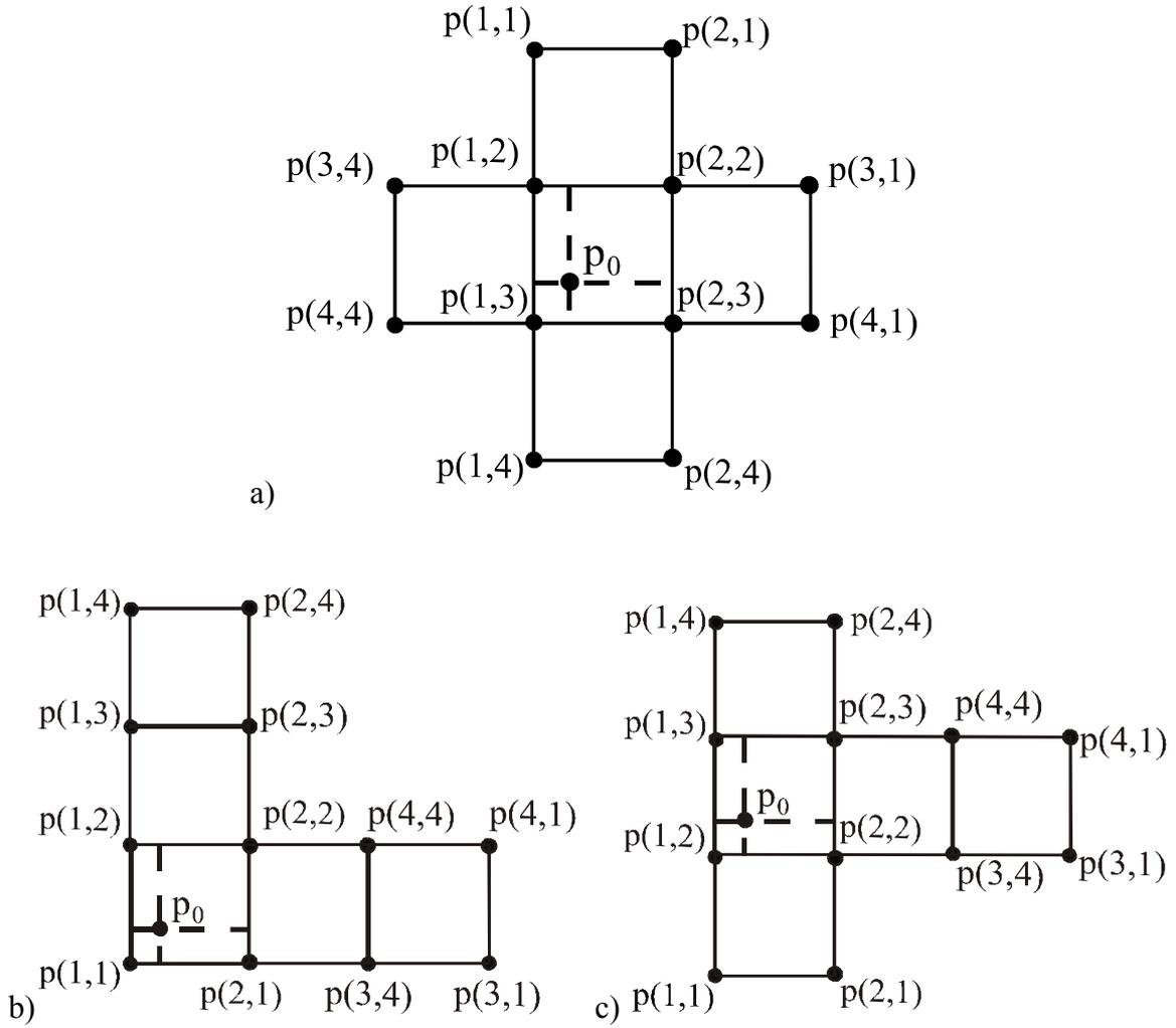
**Figure A2.** Intersecting lines for interpolation with twelve points. Location of the interpolated point ( $P'_0$ ).
