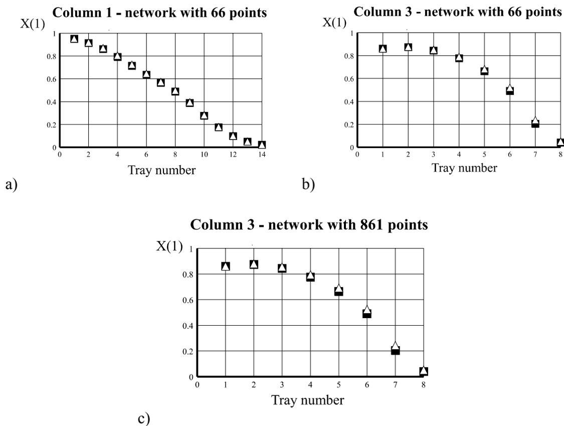
**Figure 10.** Comparison between the rigorous design method (■) and the approximate method (Δ) using a network with 66 (a-b) and 861 (c) points and the interpolation by intercepting lines from the 12 nearest points and the intersection procedure proposed, for cases 1 (a) and 3 (b-c).
