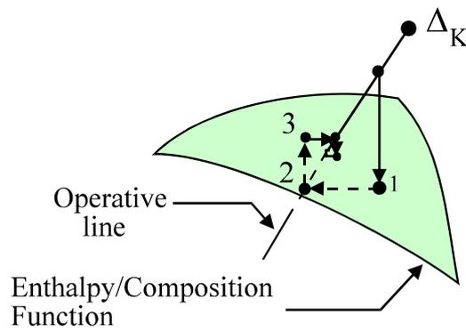
**Figure D1.** Sketch of the iterative calculation to determine the intersection point between an operative line and the enthalpy-composition surface
