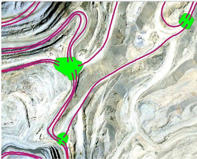
Fig. 9. Roads and context areas are overlaid on a aerial image of the mine site. The important context areas in this image are the intersections, particularly the large, four-way intersection in the center of the image.
