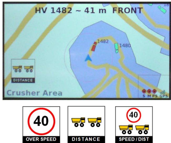
Fig. 11. Display implementation currently installed in mining vehicles. The context area name can be seen in the bottom left of screen. Several warning icons representing breaches of the rules are presented.
