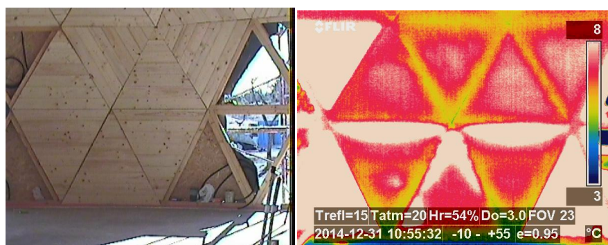
Figure 22. Image of the deformation of the cellulose inside the enclosure.
