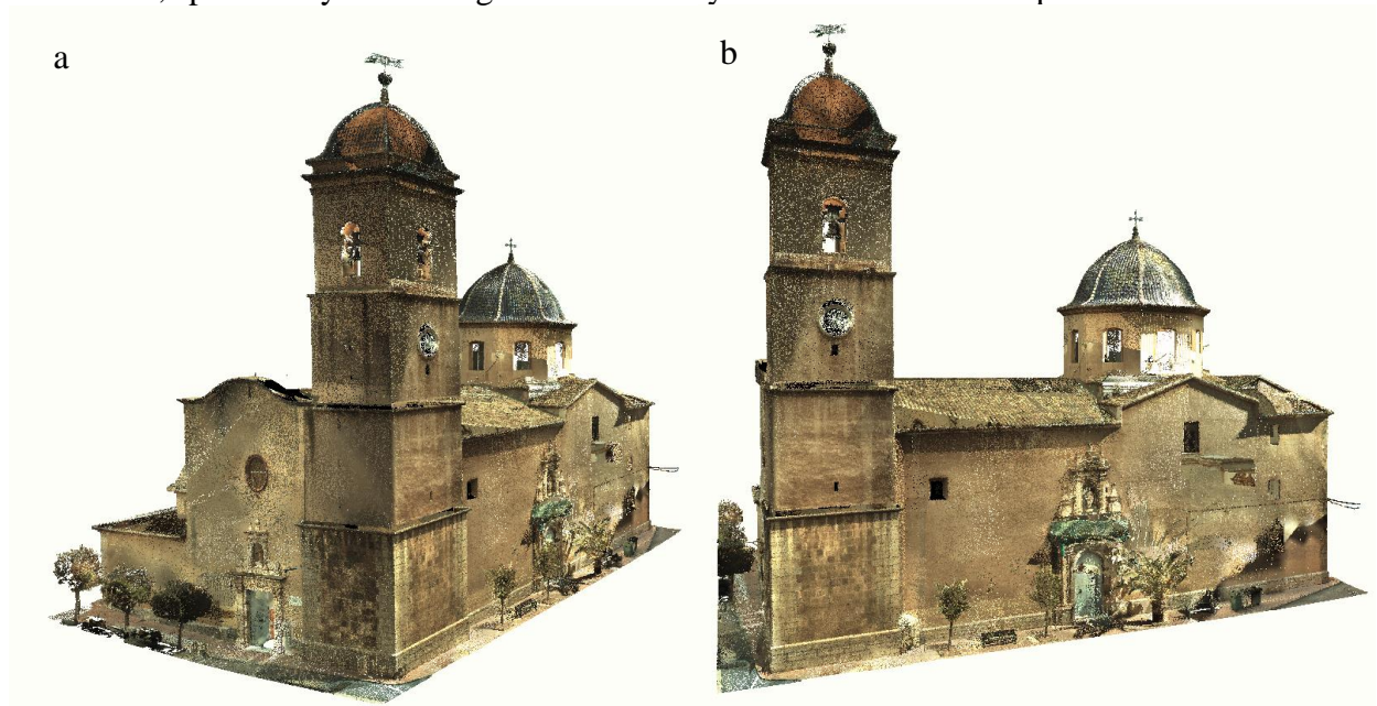
Figure 1. Main façades of the church obtained by topographic survey with Laser-Scanner. (a) Main entrance, (b) Façade of San Pedro.
