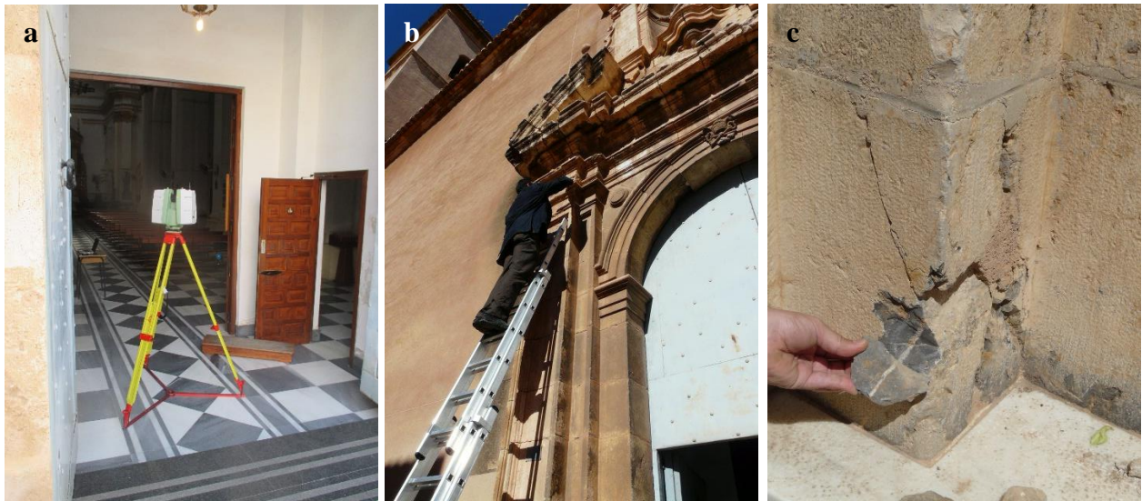
Figure 4. Different aspects of data and sample collection. a) Detail of geometric recording with laser scanner. b) Collection of samples of loose fragments on the cornice. c) Black stone flake in lower corner for observation.
