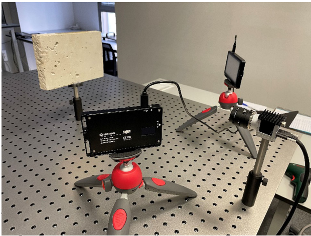
Fig. 2 Setup for the experiments. In the image, a concrete texture is being recorded
