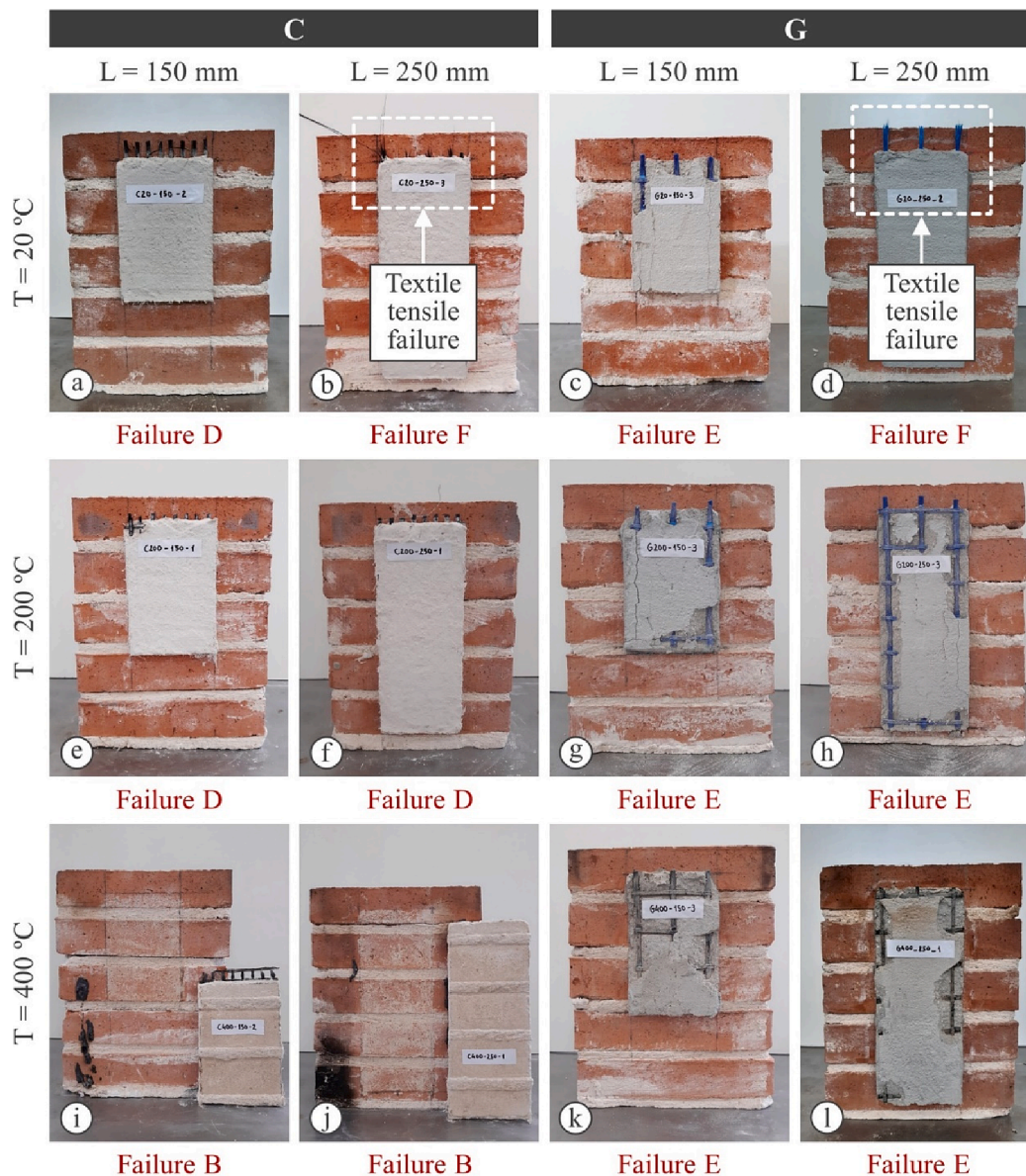
Fig. 8. Failure modes obtained in all series (meshes were cut manually after testing, except in case of textile tensile failures).
