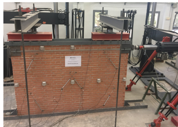
Fig. 5. Accelerometers configuration during dynamic test of the masonry wall.
