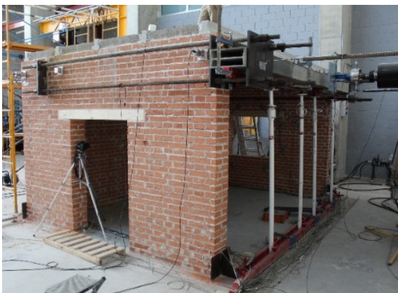
Fig. 2. Accelerometers configuration during dynamic test of simple clay brick construction.
