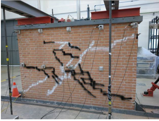
Fig. 9. Damage pattern during the test of masonry wall.
