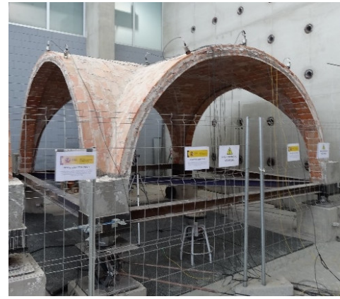
Fig. 4. Accelerometers configuration during dynamic test of the cross vault.
