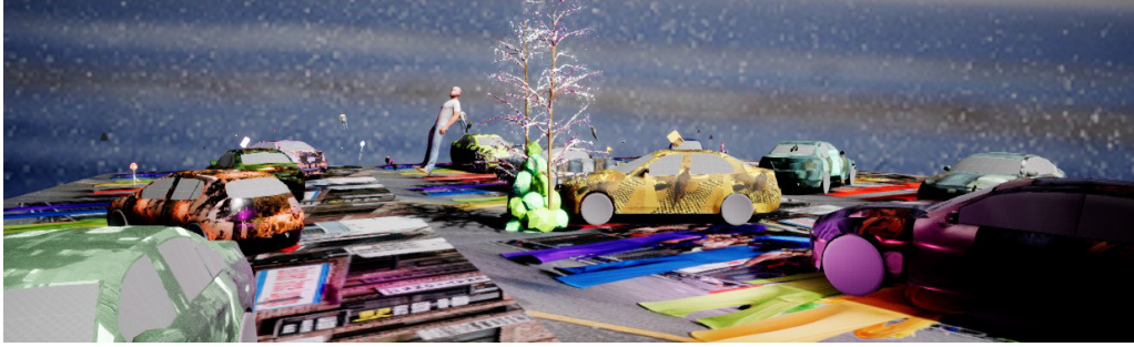
Figure 2.10: Domain randomization intentionally avoids photorealism for variety, which leads to weird generated synthetic data [Pra18].
