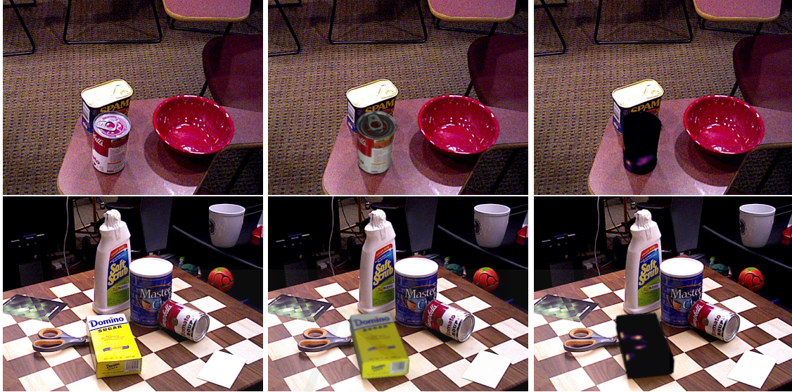
Figure 3.7: Two sample frames from the YCB Video dataset, on the top we focus on the tomato soup can , and on the bottom we focus on the sugar box . On left, the RGB images. In the middle, the synthetic 3D model of the object projected in the image with the same 6D pose. On right, the synthetic 3D model with the SynContact heat map texture.
