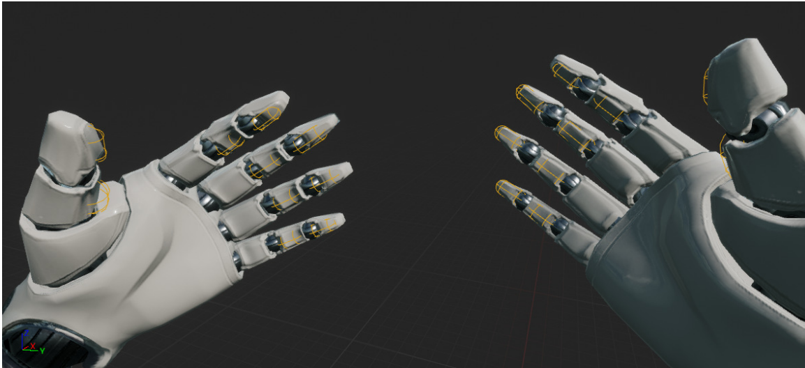
Figure 2.26: Sphere trigger volumes placed on finger phalanges of both hands represented in yellow.
