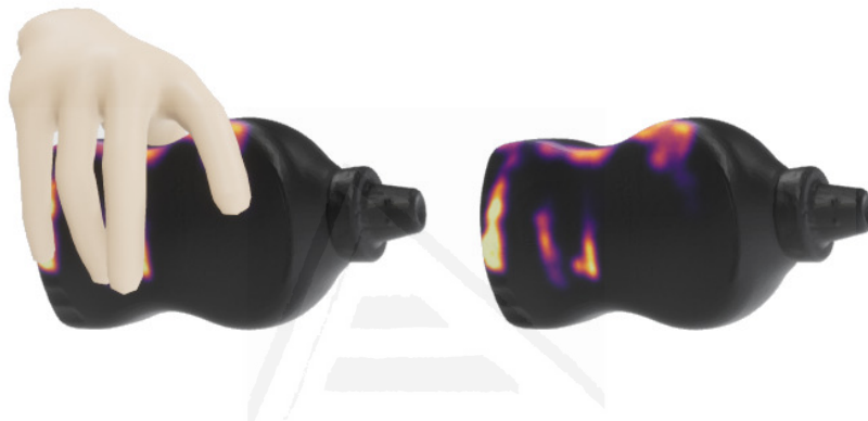
Figure 3.1: At left, a virtual hand grabbing the mustard bottle from YCB object dataset; at right, a generated contact map on the mustard bottle.
