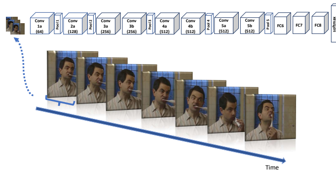
Figure 6. This figure illustrates the OAD-3D-CNN model that is used to monitor patients’ daily living activities. The AI model is fed with the video stream captured by the camera installed on the LOLA platform. In particular, clips of 16 contiguous video frames are passed to the model. Eight 3D convolutions are included in the deep learning architecture, followed by five max-pooling layers and three fully connected layers. A final softmax layer is responsible for producing the classification of the action for every video clip.
