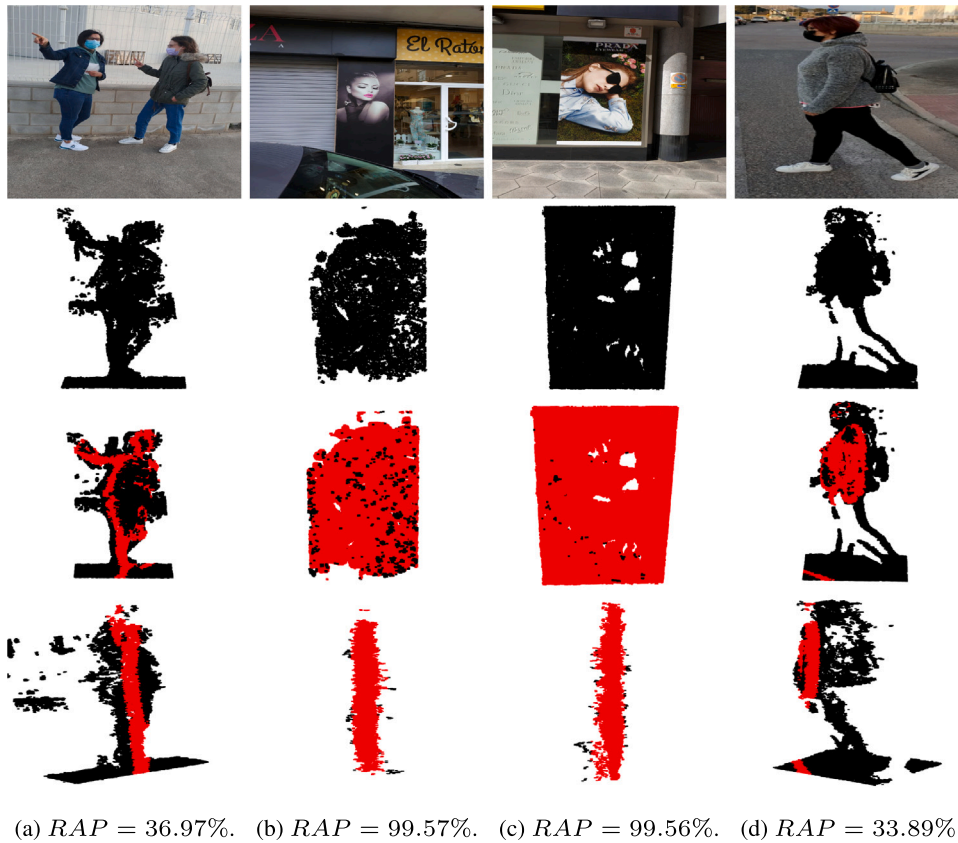
Fig. 9. (First row) Images from four random image sequences obtained by the real camera from the Custom Real Dataset 4.2. (Second row) SfM reconstructions from the image sequences that contain the top row image samples. (Third row) Front-view of RANSAC plane calculations colored in red over the SfM 3D reconstruction in black. (Fourth row) Side-view of RANSAC plane calculations colored in red over the SfM 3D reconstruction in black.
