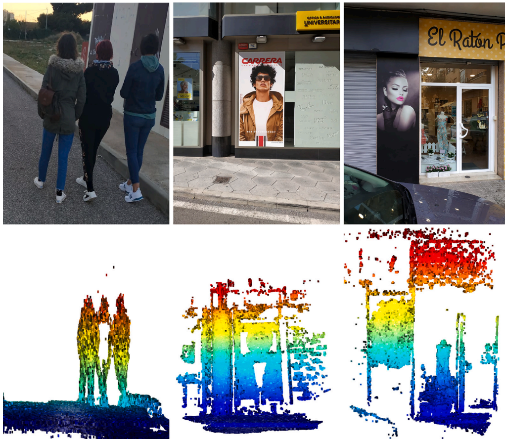
Fig. 2. The top row depicts images from three random image sequences obtained by the camera that are used to perform the scene reconstruction. The bottom row shows SfM reconstructions from the images sequences that contain the top row image samples.
