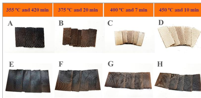
**Figure 6.** Thermal degradation over time of resin within a unique non-submerged part of a solid residue from the HTD process (R\_23) differentiating between the smallest size of 0.50 cm  $\times$  1.65 cm (A,B,C, and D) and the biggest size of 3.30 cm  $\times$  4.00 cm (E,F,G, and H) used in this work when using a scaling program temperature from 355 to 450 °C according to the neutral scenario.
