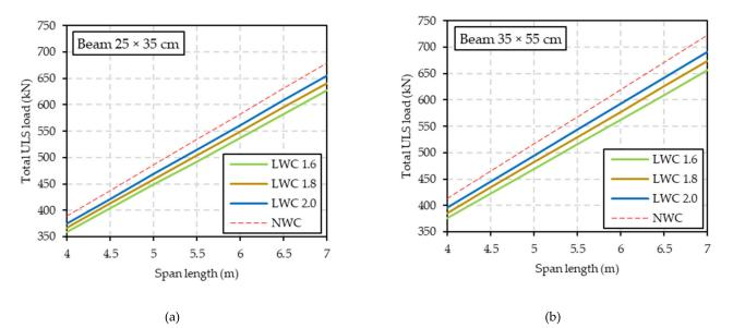
**Figure 7.** Total ULS design load upon the three beam supports, with  $q_{live} = 2 \text{ kN/m}^2$ , TW = 4.5 m and d' = 4 cm (regardless of concrete strength, cement type and redistribution factor  $\delta$ ): (a) downstand beam with dimensions  $b \times h = 25 \times 35 \text{ cm}$ ; (b)  $b \times h = 35 \times 55 \text{ cm}$ .
