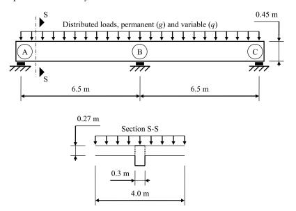
Figure 4. Two-span reinforced concrete beam.
