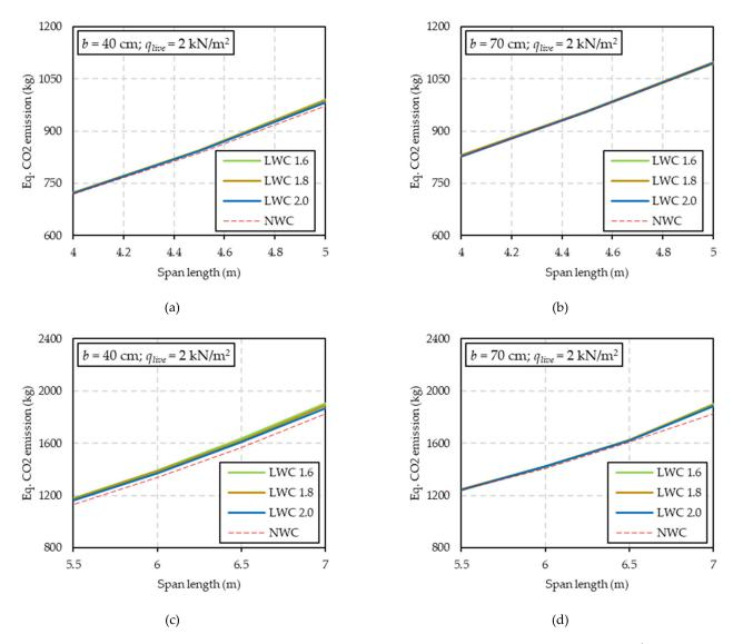
**Figure 15.** Estimated CO<sub>2</sub> emissions by flat beams made with  $f_{(l)ck} = 30$  MPa concrete (with CEM 42.5), with d' = 3.5 cm, supporting a live load  $q_{live} = 2 \text{ kN/m}^2$  with TW = 4.5 m and designed with  $\delta = 0.85$ : (**a**,**b**) span L = 4-to-5 m; (**c**,**d**) L = 5.5-to-7 m; (**a**,**c**) cross-sectional width b = 40 cm; (**b**,**d**) width b = 70 cm.
