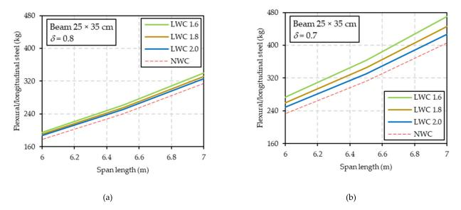
**Figure 9.** Total mass of longitudinal steel reinforcements along the continuous beam, with  $q_{live} = 2 \text{ kN/m}^2$ , TW = 4.5 m, d' = 4 cm and  $f_{ck}$  ( $f_{lck}$ ) = 25 MPa (regardless of cement type): (a) beam with  $b \times h = 25 \times 35$  cm and  $\delta = 0.8$ ; (b)  $b \times h = 35 \times 55$  cm and  $\delta = 0.7$ .
