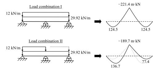
**Figure 5.** Load combinations and bending moment diagrams in the LWC beam made with density class 1.8, with linear elastic analysis and  $\delta$  = 1.
