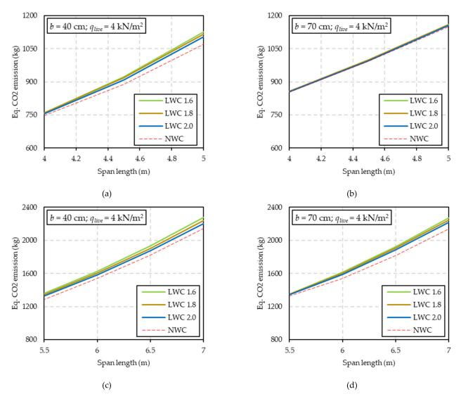
**Figure 16.** Estimated CO<sub>2</sub> emissions by flat beams made with  $f_{(l)ck} = 30$  MPa concrete (with CEM 42.5), with d' = 3.5 cm, supporting a live load  $q_{live} = 4$  kN/m<sup>2</sup> with TW = 4.5 m and designed with  $\delta = 0.85$ : (**a**,**b**) span L = 4-to-5 m; (**c**,**d**) L = 5.5-to-7 m; (**a**,**c**) cross-sectional width b = 40 cm; (**b**,**d**) width b = 70 cm.
