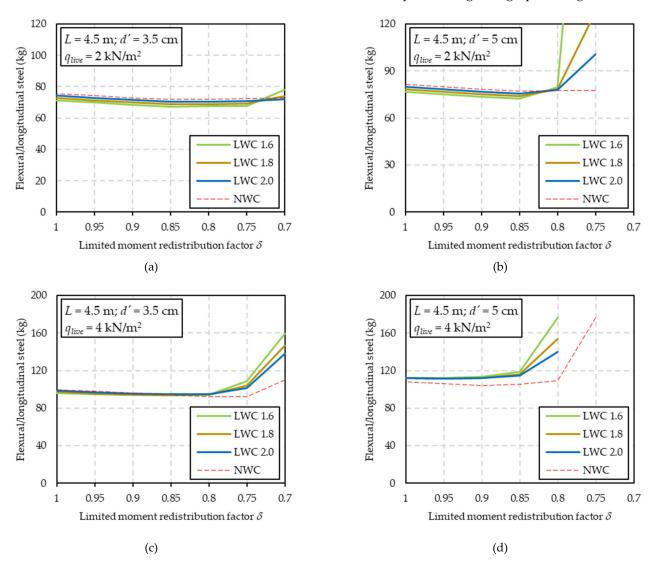
**Figure 14.** Reinforcing steel required by flat beams (b = 55 cm) made with  $f_{(l)ck} = 30$  MPa concrete (with CEM 42.5), supporting a TW = 4.5 m, with L = 4.5 m: (**a**,**b**)  $q_{live} = 2$  kN/m<sup>2</sup>; (**c**,**d**)  $q_{live} = 4$  kN/m<sup>2</sup>; (**a**,**c**) d' = 3.5 cm; (**b**,**d**) d' = 5 cm.
