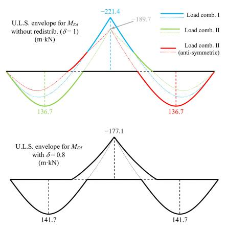
**Figure 6.** ULS envelopes of bending moments in the LWC beam made density class 1.8, when  $\delta = 1$  and when  $\delta = 0.8$ .
