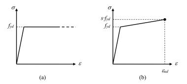
**Figure 3.** Bi-linear stress–strain distribution of reinforcing steel for ULS design: (**a**) without plastic hardening nor tensile strain limitation; (**b**) with plastic hardening and tensile strain limitation.
