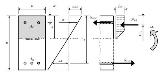
Figure 2. Rectangular reinforced lightweight aggregate concrete cross-section subjected to pure bending.
