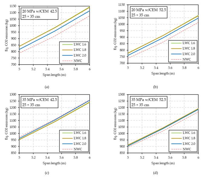
**Figure 10.** Estimation of CO<sub>2</sub> emission on account of cement and steel consumption by  $25 \times 35$  cm ( $b \times h$ ) beams with  $q_{live} = 2 \text{ kN/m}^2$ , TW = 4.5 m, d' = 4 cm: (**a**,**c**) CEM 42.5; (**b**,**d**) CEM 52.5; (**a**,**b**)  $f_{ck} = f_{lck} = 20 \text{ MPa}$ ; (**c**,**d**)  $f_{ck} = f_{lck} = 35 \text{ MPa}$ .
