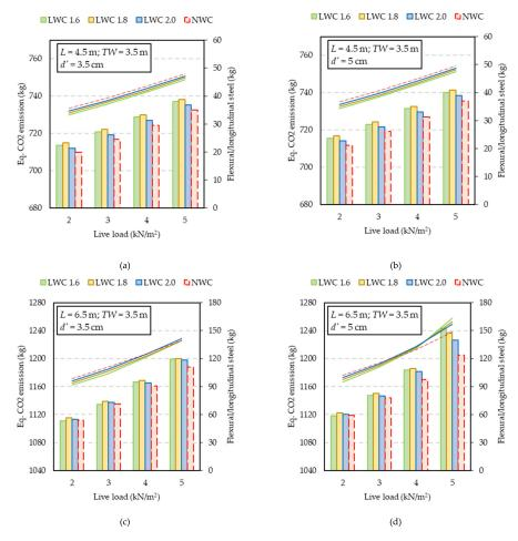
**Figure 12.** Estimation of CO<sub>2</sub> emission (cement + steel) and mass of reinforcing steel in  $30 \times 45$  cm ( $b \times h$ ) beams made with  $f_{(l)ck} = 30$  MPa concrete (with CEM 42.5). Global analysis with  $\delta = 0.8$  and slab tributary width TW = 3.5 m: (**a**,**b**) span L = 4.5 m; (**c**,**d**) span L = 6.5 m; (**a**,**c**) concrete cover d' = 3.5 cm; (**b**,**d**) concrete cover d' = 5 cm.
