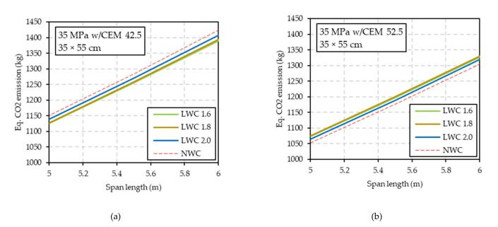
**Figure 11.** Estimation of CO<sub>2</sub> emission on account of cement and steel consumption by  $35 \times 55$  cm ( $b \times h$ ) beams with  $q_{live} = 2 \text{ kN/m}^2$ , TW = 4.5 m, d' = 4 cm,  $f_{ck} = f_{lck} = 35 \text{ MPa}$ : (**a**) 35 MPa concrete made with CEM 42.5; (**b**) 35 MPa concrete made with CEM 52.5.
