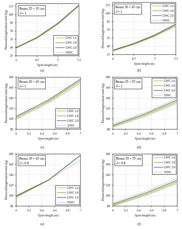
**Figure 8.** Total mass of longitudinal steel reinforcements along the continuous beam, with  $q_{live} = 2 \text{ kN/m}^2$ , TW = 4.5 m, d' = 4 cm and  $f_{ck}$  ( $f_{lck}$ ) = 25 MPa (regardless of cement type): (**a**–**d**) with  $\delta = 1$ ; (**e**,**f**) with  $\delta = 0.8$ ; (**a**) downstand beam with dimensions  $b \times h = 25 \times 35 \text{ cm}$ ; (**b**,**c**,**e**)  $b \times h = 30 \times 45 \text{ cm}$ ; (**d**,**f**)  $b \times h = 35 \times 55 \text{ cm}$ .
