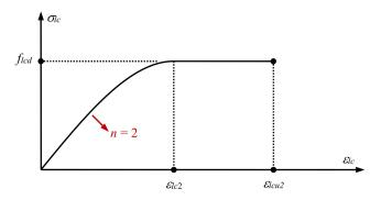
Figure 1. Parabola-rectangle diagram for normal strength lightweight aggregate concrete.
