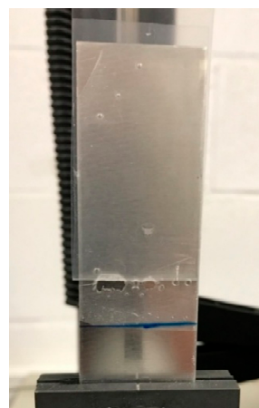
Figure 10. Loci of failure of aluminum 5754/TPU PSA joints.
