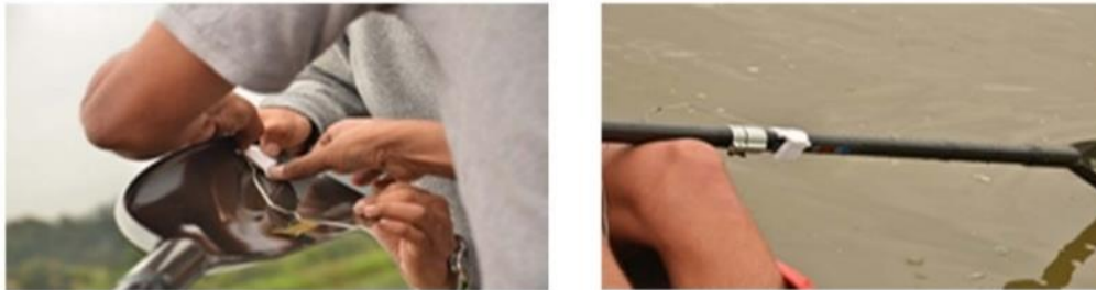
Figure 1. Left. Water sensor. Right. Motion sensor of the paddle
