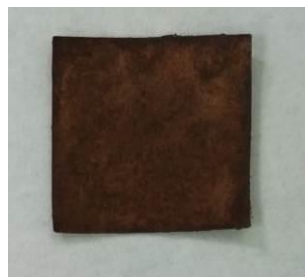
Figure. Magnetic paper-based sorptive phases based on the coating of a paper substrate by a magnetic nanocomposite.
