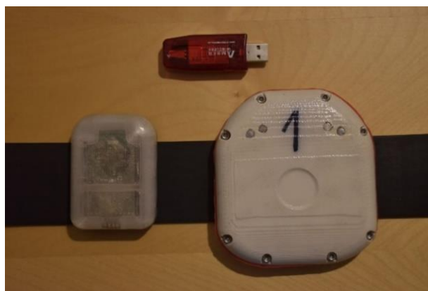
Figure 2. Larger version of IMU 1 (right) and a new smaller reduced version of IMU (left) and USB RF receiver (top).
