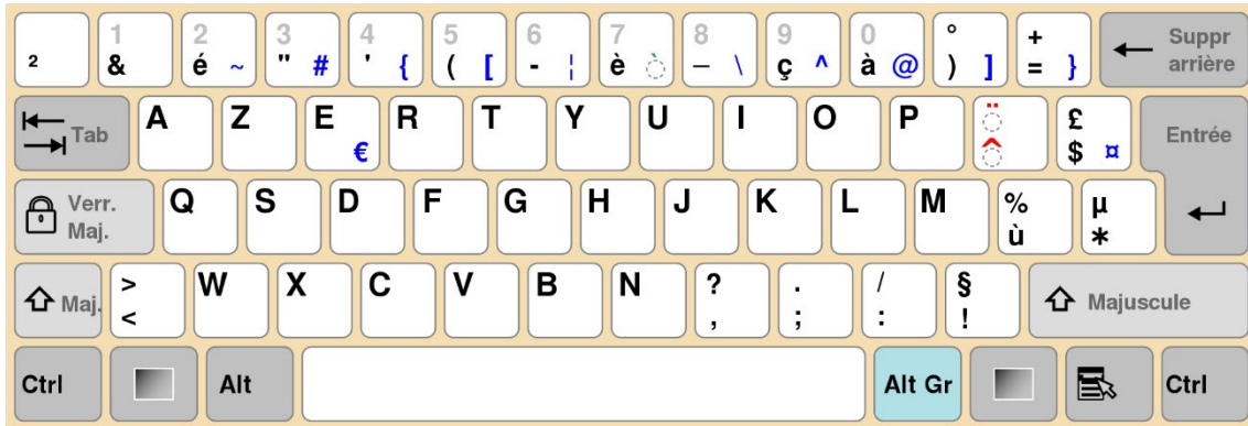
Fig. 2 – AZERTY (France) Keyboard layout 13 . Dead keys appear in red color and characters obtained by pressing “Alt Gr” simultaneously appear in blue and the sole case of both “¨” (dead key + “Alt Gr”) appears in green.
