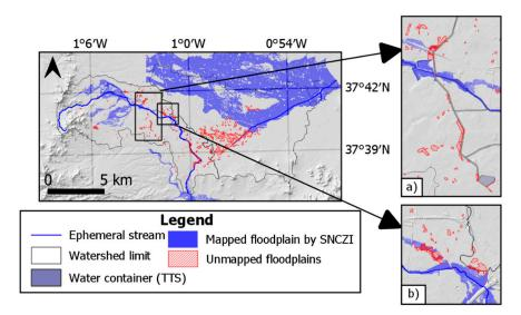
**Figure 17.** Flood-prone areas caused by human intervention: (**a**) shows floodable areas produced by terrain modifications made to mitigate the lack of fluvial connectivity caused by the Tagus-Segura Transfer (TTS) water channel; in the case of (**b**) irrigated crops under plastic produce a large extension of water during floods.
