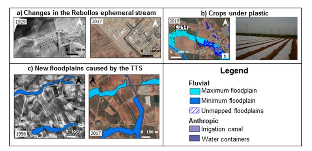
**Figure 15.** Human interventions that alter flooding in the Rebollos watershed. (**a**) the Rebollos ephemeral stream disappears due to the terrain modification to an industrial estate, (**b**) flow rate and exposure increase as a result of the use of plastic on crops, and (**c**) loss of floodplain connectivity, and consequently, increased exposure of new areas to flooding.
