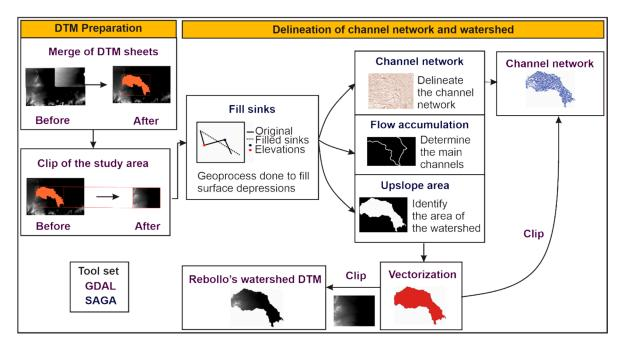
Figure 4. Geoprocess to delineate and describe the channel networks and watershed.
