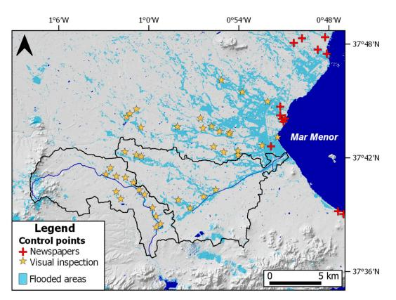
**Figure 6.** Control points to determine flood threshold. Data were based on newspaper articles and visual inspection from RGB bands of Sentinel-2 satellite images.
