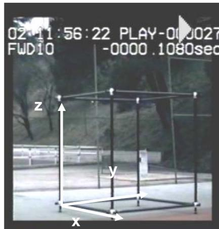
**Figure 2.** Calibration Object
