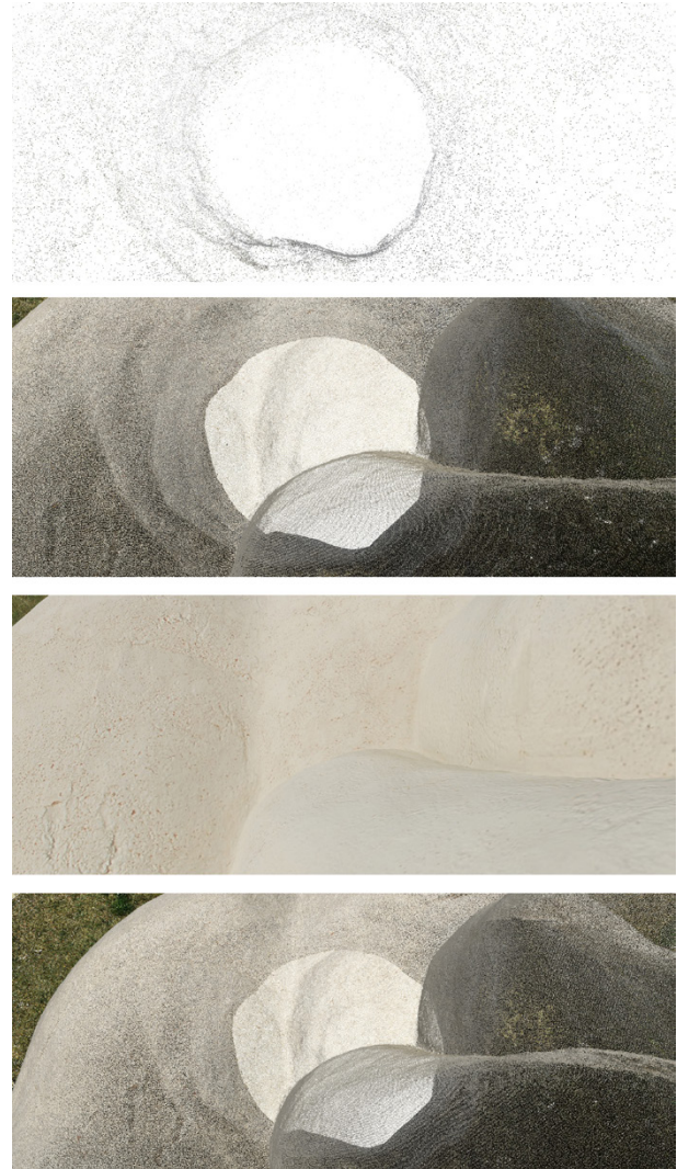
Fig. 2. Top to bottom, the classic workflow in a photogrammetry program: point detection to orient photos, dense point cloud, textured and Meshed surfaces and overlapping.
