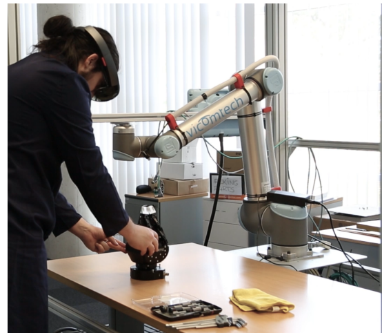
Figure 2: An operator using the AREVA system to carry out the gripper's maintenance
