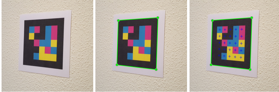
Figure 7: Original image (left). Result of the frame detection algorithm (center). N \times N grid obtained from frame coordinates.
