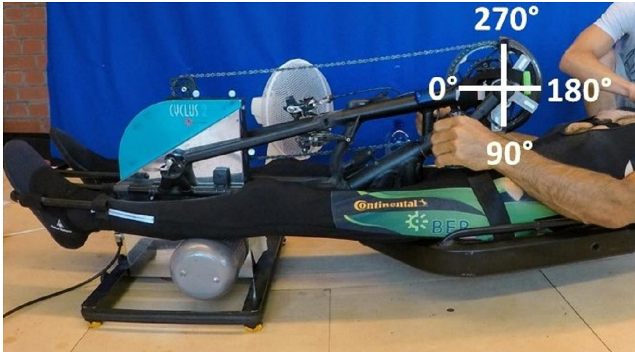
Figure 1. The test set-up with the recumbent arm power bike mounted on the Cyclus2 ergometer. The crank position was defined along the horizontal 0-180° axis. A hip belt was used to stabilize the participants on the bike.
