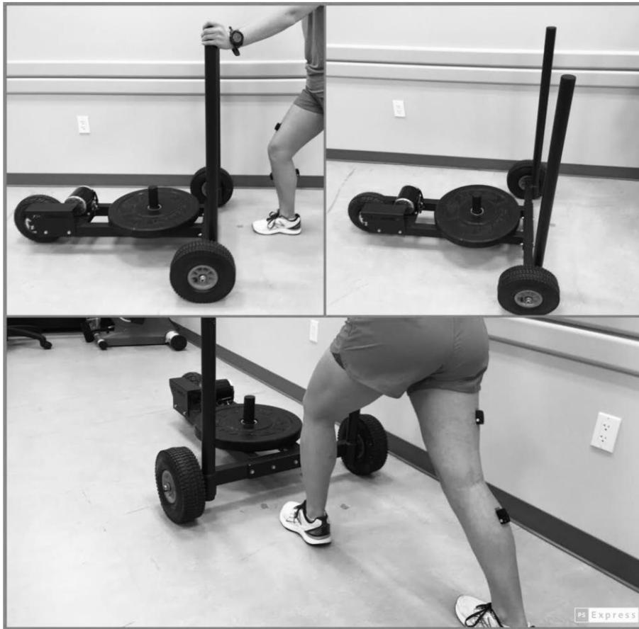
Figure 1. Sled XPO Trainer with surface EMG electrode placement on Tibialis Anterior, Gastrocnemius, Hamstring and Quadriceps.
